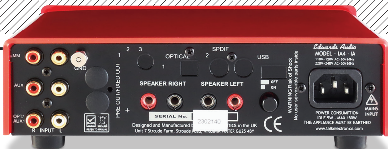
ABOVE: Two line inputs and an MM phono, all on RCA, are hosted adjacent to blanked-off inputs for a preamp output and forthcoming/optional digital modules. Speaker outputs are on PCB-mounted 4mm sockets for banana plugs only
