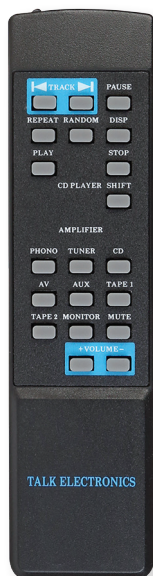
LEFT: Talk-branded remote offers control over the IA1's input selection, motorised volume and mute
